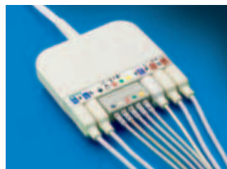
CombiCable: EKG/RESP, ST and arrhythmia analysis, SpO 2 , 2 x IBP and 2 x TEMP with one connection port to the monitor
