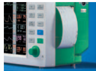
Optional integrated recorder 5) for documentation: 6-channel thermal recorder with excellent printing quality.
